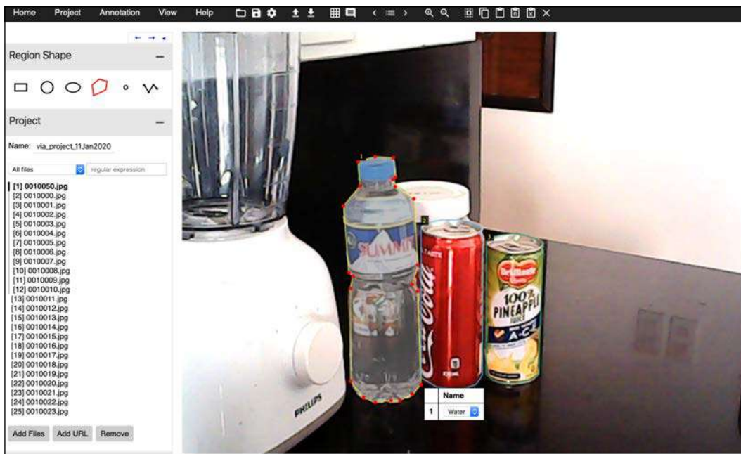
Figure 12.4.1: Dataset labeling process for semantic segmentation using the VGG Image Annotator (VIA)
